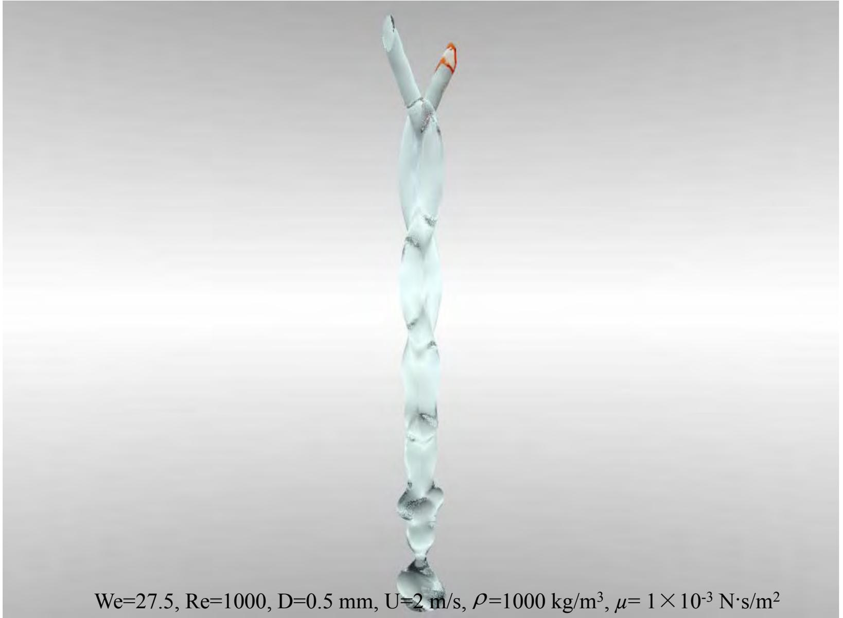
$We=27.5$ ,  $Re=1000$ ,  $D=0.5$  mm,  $U=2$  m/s,  $\rho=1000$  kg/m<sup>3</sup>,  $\mu=1 \times 10^{-3}$  N·s/m<sup>2</sup>
